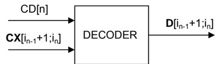
Figure H.5 – Bit clock based JPEG 2000 Part 1 arithmetic decoder.
