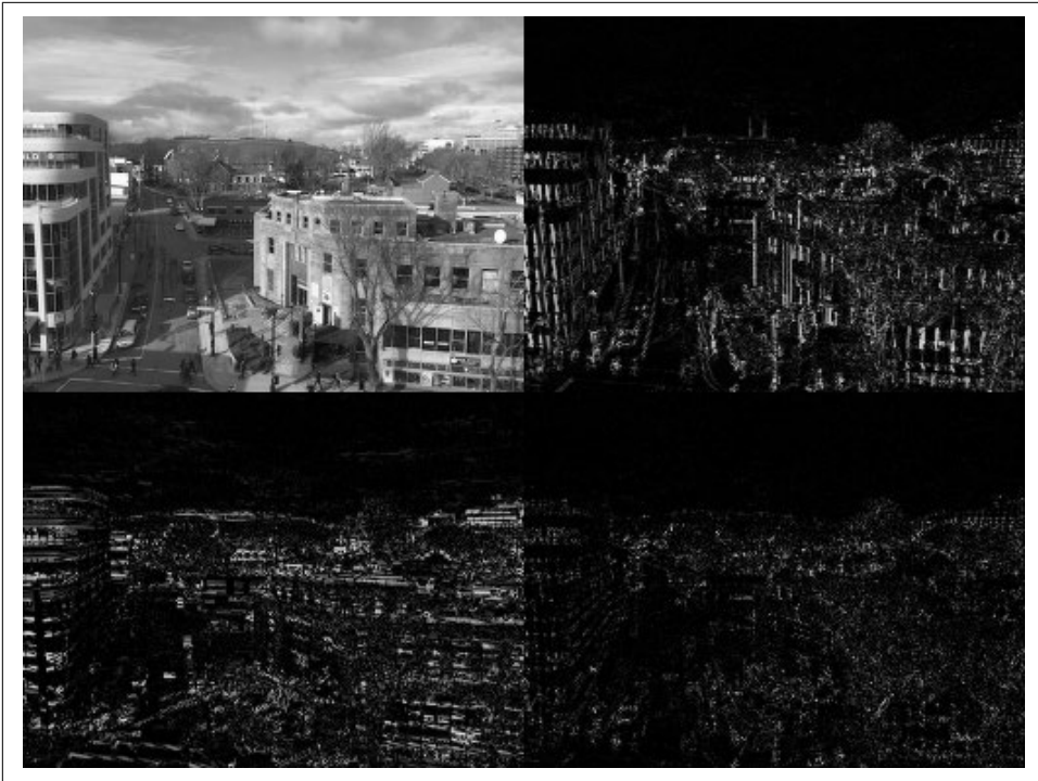
Figure 5-2. Image after Discrete Wavelet Transform (details enhanced for demonstration purposes)
