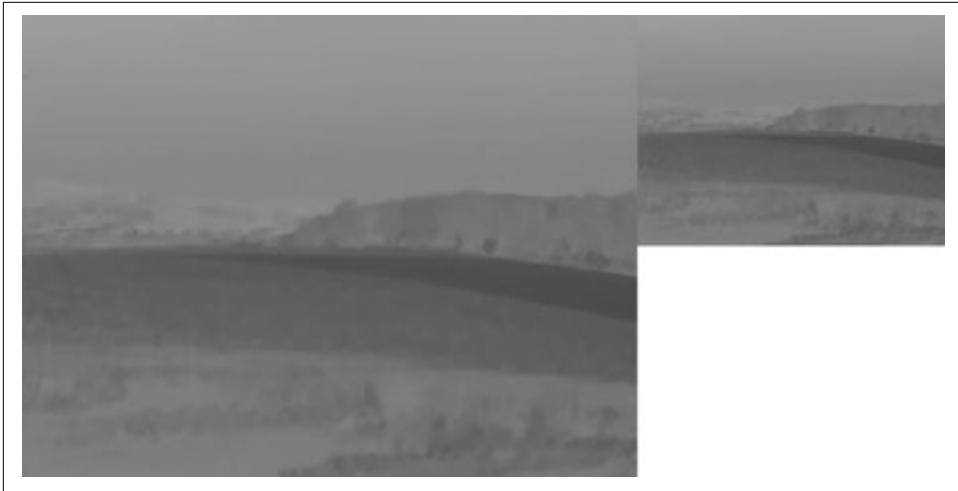
Figure 4-4. To the left, the original (untaunted) Cb component. To the right, the same component after 4:2:0 subsampling
