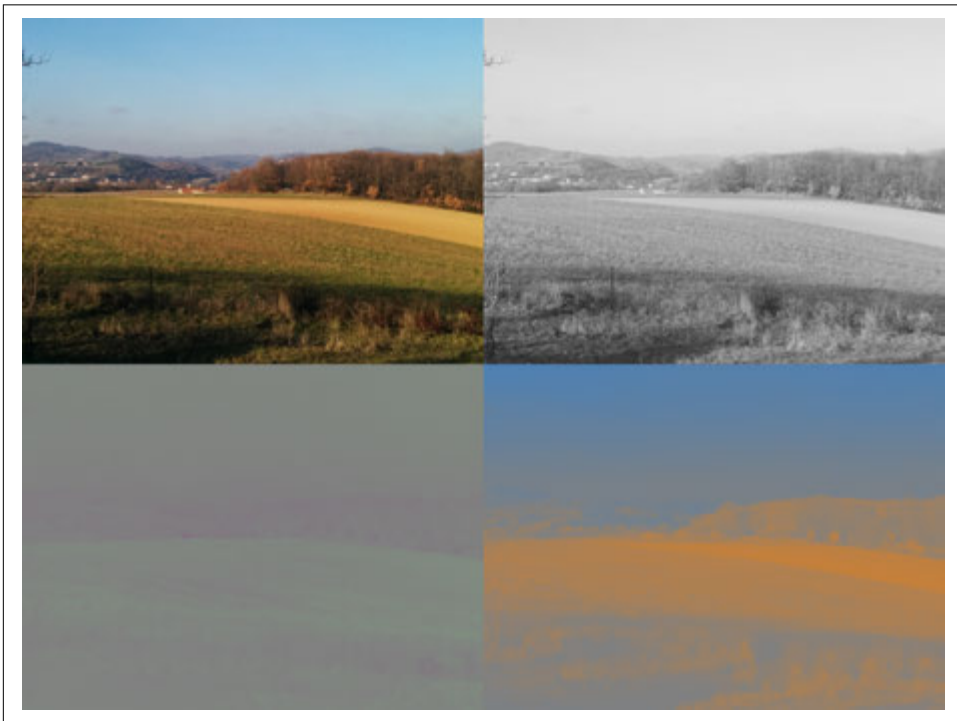
Figure 2-9. Winter-time French countryside. Top to bottom, left to right: Full image, Y component, Cg component and Co component.
