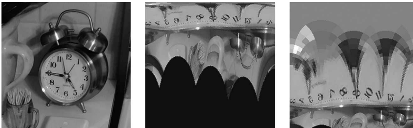
Figure 6.12 (a) The original image, (b) the radial-polar transformation of the image, and (c) the log-polar transformation.
