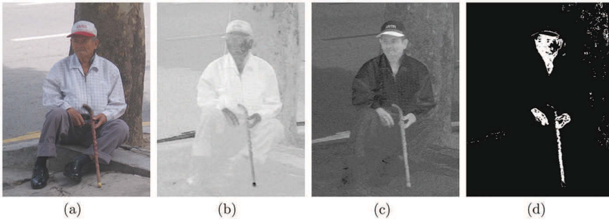
Figure 2.2 (a) An original image, (b) the I channel from the YIQ color model, (c) the Q channel, and (d) pixels that passed both thresholds.
