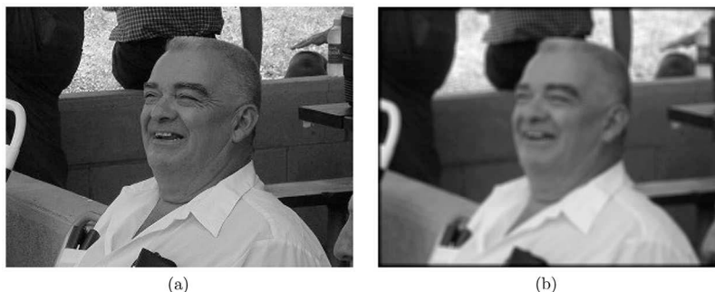
Figure 12.2 (a) The original image and (b) the image after correlation with a small solid block (Code 12.1).
