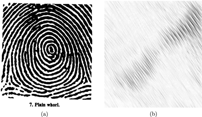
Figure 11.5 (a) A fingerprint and (b) the negative of the result after the application of the wedge filter shown in Figure 11.3.
