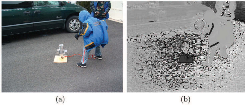
Figure 5.7 (a) An image with a gray drive and (b) the hue channel depicting widely varying values in the gray regions.
