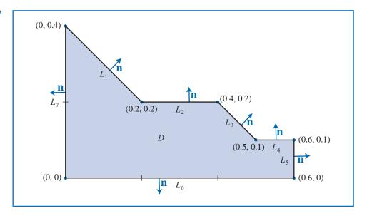
We first subdivide D into triangles with the labeling suggested in Step 0 of the algorithm. For this example,  $S_1 = L_6 \cup L_7$  and  $S_2 = L_1 \cup L_2 \cup L_3 \cup L_4 \cup L_5$ . The labeling of triangles is shown in Figure 12.18.
