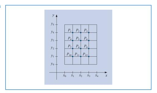
**Example 1** Determine the steady-state heat distribution in a thin square metal plate with dimensions 0.5 m by 0.5 m using n = m = 4. Two adjacent boundaries are held at 0°C, and the heat on the other boundaries increases linearly from 0°C at one corner to 100°C where the sides meet.
