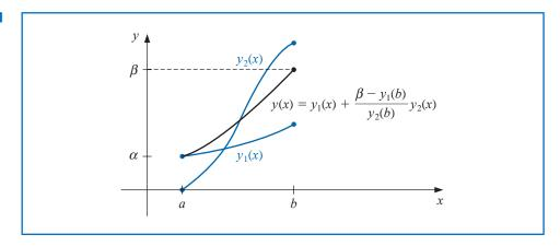
Algorithm 11.1 uses the fourth-order Runge-Kutta technique to find the approximations to  $y_1(x)$  and  $y_2(x)$ , but other techniques for approximating the solutions to initial-value problems can be substituted into Step 4.
