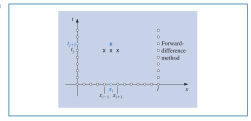
**Example 1** Use steps sizes (a) h = 0.1 and k = 0.0005 and (b) h = 0.1 and k = 0.01 to approximate the solution to the heat equation
