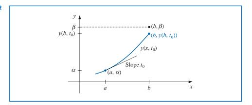
If  $y(b, t_0)$  is not sufficiently close to  $\beta$ , we correct our approximation by choosing elevations  $t_1, t_2$ , and so on, until  $y(b, t_k)$  is sufficiently close to "hitting"  $\beta$ . (See Figure 11.3.)
