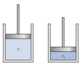
We then repeat the experiment using the same values of R and N, but increase the pressure by a factor of two and reduce the volume by the same factor. The product PV remains the same, so the predicted temperature is still 17°C. But now we find that the actual temperature of the gas is 19°C.
