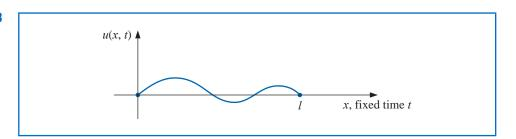
If the string is set to vibrate in a vertical plane, the vertical displacement u(x, t) of a point x at time t satisfies the partial differential equation
