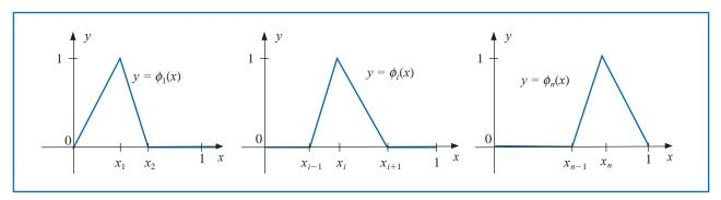
The functions  $\phi_i$  are piecewise-linear, so the derivatives  $\phi'_i$ , while not continuous, are constant on  $(x_i, x_{i+1})$ , for each j = 0, 1, ..., n, and
