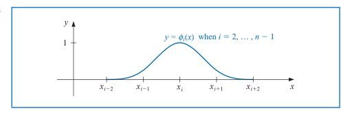
Since  $\phi_i(x)$  and  $\phi'_i(x)$  are nonzero only for  $x \in [x_{i-2}, x_{i+2}]$ , the matrix in the Rayleigh-Ritz approximation is a band matrix with bandwidth at most seven:
