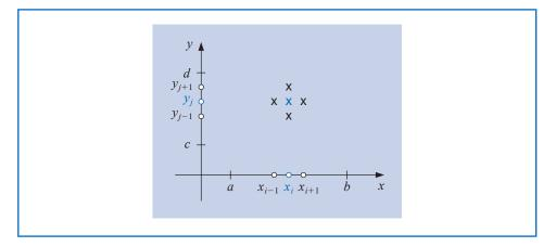
We use the information from the boundary conditions (12.5) whenever appropriate in the system given by (12.4); that is, at all points  $(x_i, y_i)$  adjacent to a boundary mesh point.
