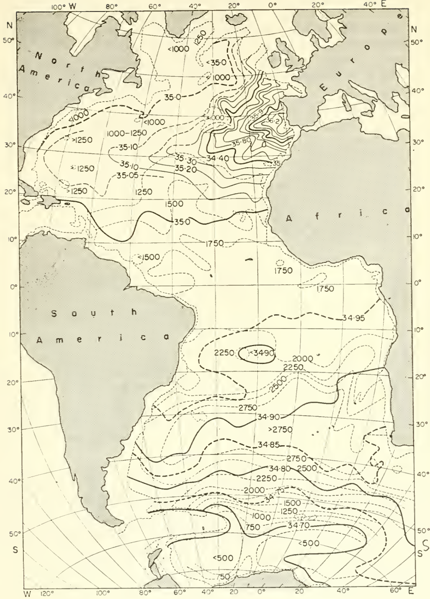
FIG. 329. Spreading and depth of the upper North Atlantic Deep Water (Mediterranean Water). The thin dashed lines indicate the depth of the core layer in metres (according to Wüst).
