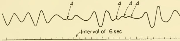
FIG. 22. Registration of a wave train by a wave recorder of the Admiralty.
