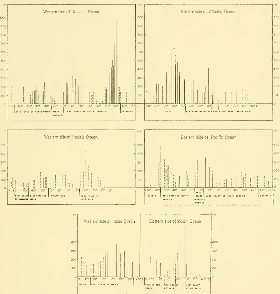
CHART III. Average range at springtide of semi-diurnal tides 2(M_2 + S_2) in centimetres. The character of tide F = \frac{(K_1 + O_1)}{(M_2 + S_2)} is designated by —————: 0 < F < 0.25 semi-diurnal tides; - - - - -: 0.25 < F < 1.5 mixed, mainly semi-diurnal tides; - - - - -: 1.5 < F < 3.0 mixed, mainly diurnal tides; - - - - -: 3.0 < F < \infty diurnal tides.
