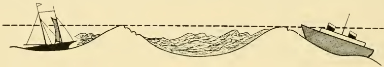
FIG. 21. Wave height measurement. (By Ch. Wilkes.)
