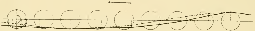
FIG. 30. — wave profile according to stereophotogrammetric pictures taken on the "Planet"; ----, trochoid of the same height; ·····, real orbit (wave height not exaggerated in height) (Kohlschütter).
