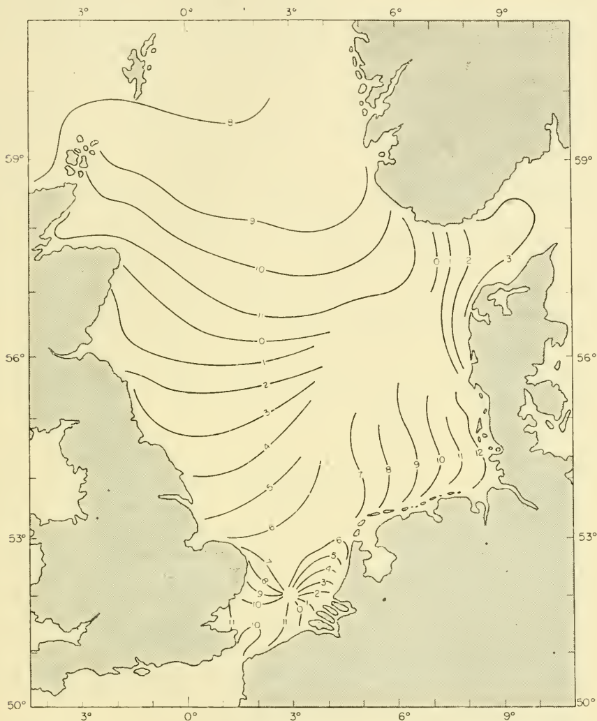
FIG. 152. Co-tidal lines of the North Sea according to Whewell. (The numbers indicate approximately the corrected establishments in lunar hours.)
