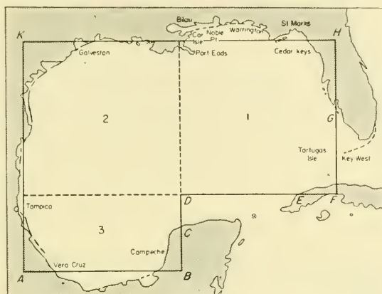
FIG. 185. Schema of the division of the Gulf of Mexico for the theoretical computation of the tides. Position of the tide stations around the Gulf.
