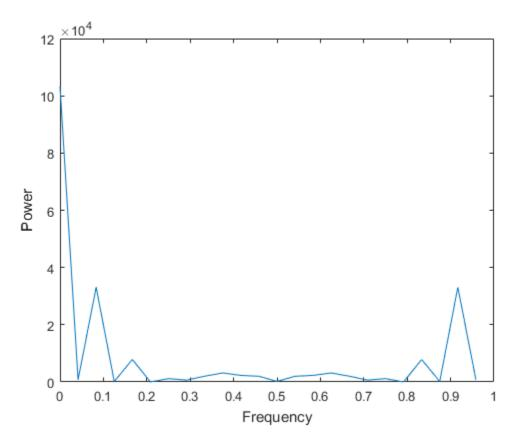
The peak near 0.0833 supports the assumption, although it occurs at a slightly higher frequency. The model can be adjusted accordingly.
