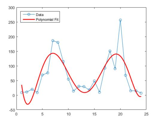
The model has the advantage of being simple while following the up-and-down trend. The accuracy of its predictive power, however, is questionable, especially at the ends of the data.
