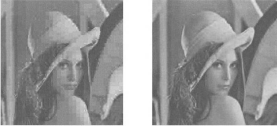
Figure 4.30. 256 \times 256 image, “Lenna,” compressed to 0.25 bps using baseline JPEG (left) and JPEG2000 (right).
