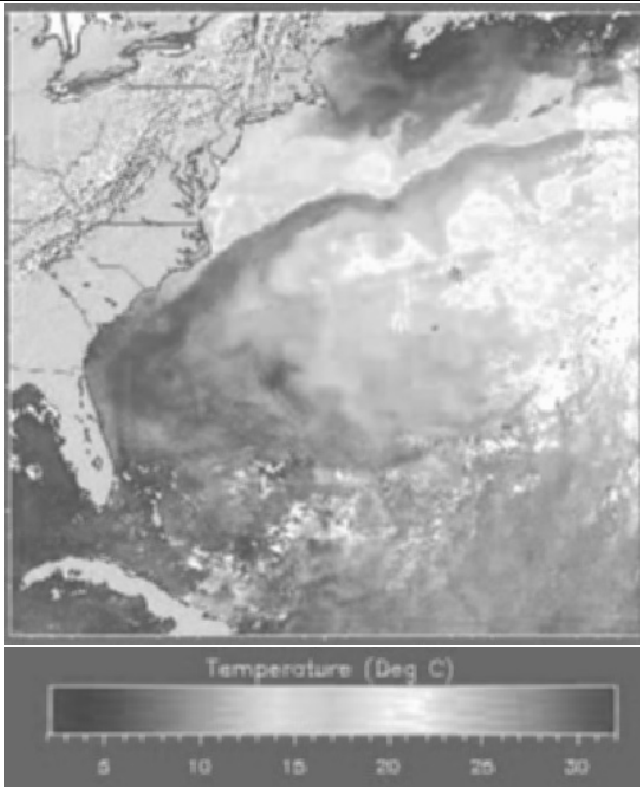
Figure 5.2. (in color on page 518). Multipass image of the SST field of the Gulf Stream region as determined by the Advanced Very High Resolution Radiometer (AVHRR) in May 1996 (obtained from http://fermi.jhuapl.edu/avhrr/gallery/sst/stream.html ).
