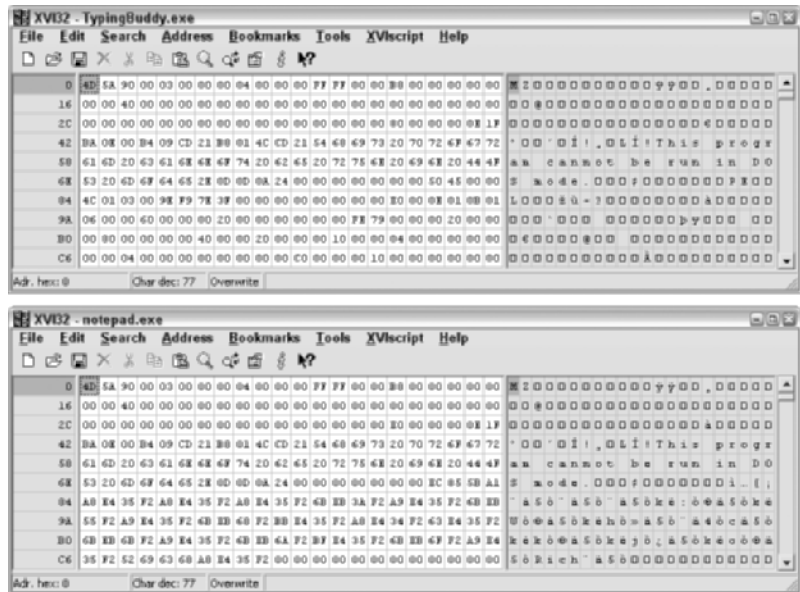
FIGURE 15.2 Hexadecimal editors can't tell the difference between .NET applications and native executables.
